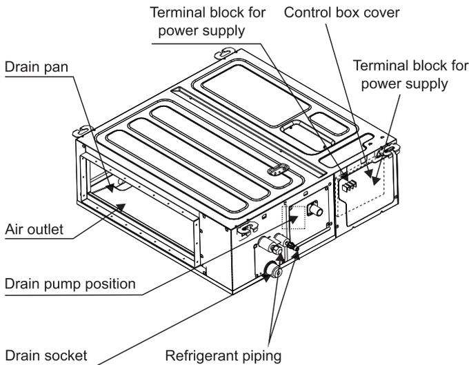
• On completion of the drainage check, refer to the following illustration, and use the provided large sealing pad and insulate the metal clamp and drain hose.
