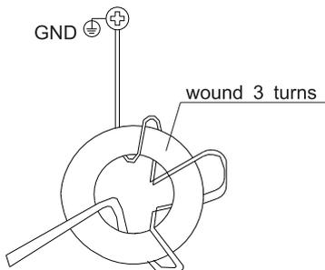
② If the model is not equipped with a wired controller, the indoor power lines L and N must be wound 3 turns with this magnetic ring, and the ground wire must be circled by another magnetic ring for 3 turns.
