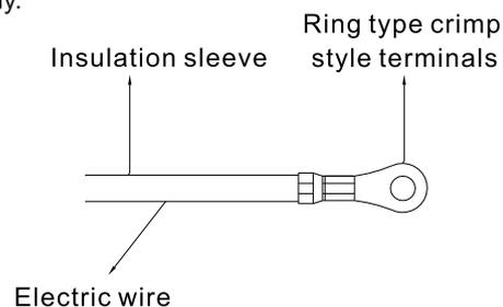
Connect wires of the same gauge to both sides.
