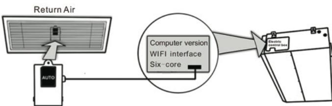
The WiFi module should be placed in the return air or some other place in WiFi area. (Customers should prepare the wireless router)
