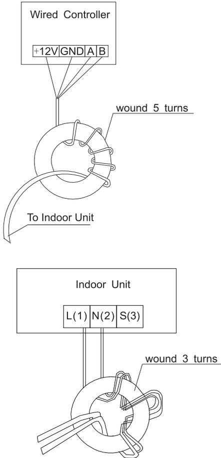
② If the model is not equipped with a wired controller, the indoor power lines L and N must be wound 3 turns with this magnetic ring.
